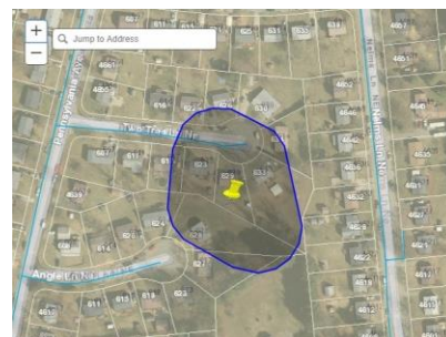
Esri map as seen on SOSRemote device. The area to be marked can be highlighted based on geo coordinates in the 811 notification.
